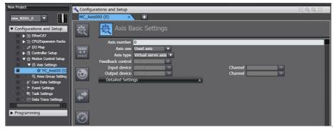
In the user program, an axis variable name is specified for the in-out variable Axis in motion control instructions.
